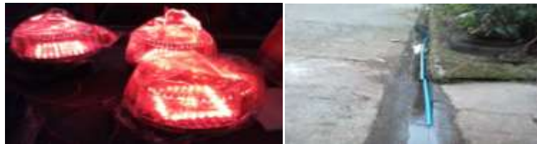
Figure 10.a Red LED Array Turns On Figure 10.b Low, Medium & High Water Level Sensors Submerged in Water
